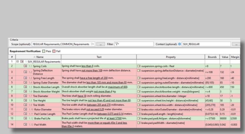
By combining text-based requirements with descriptive and analytical models in SysML, requirement verification can be automated.
